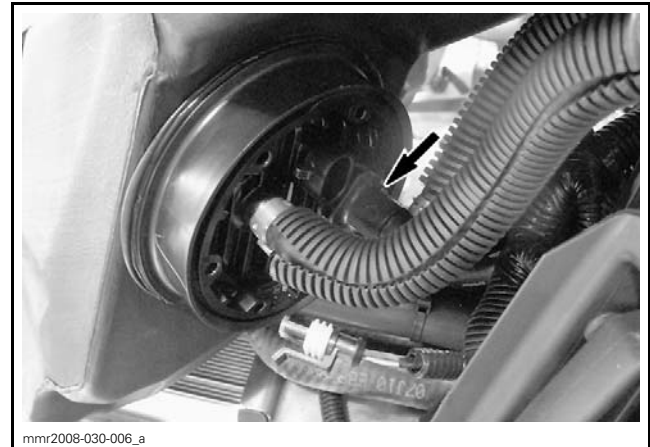
TYPICAL - FUEL SUPPLY LINE TO DISCONNECT
